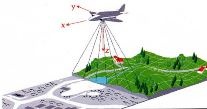
▼ Fig 1 General Principle Of Airborne Laser Scanning (ALS)
